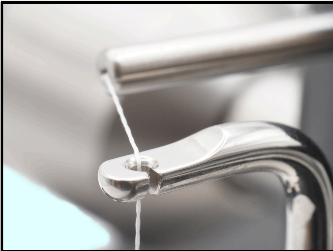
Figure–30: Fitting Anti-Skate Cord through slot in carrier arm.
