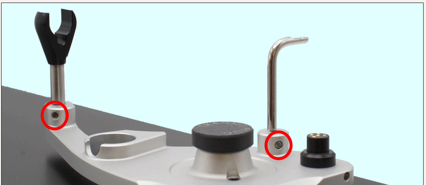
Figure–11: Showing fixing screw positions for the Anti-Skate weight arm and Tonearm support. Use the 2mm screwdriver from the tool kit.
