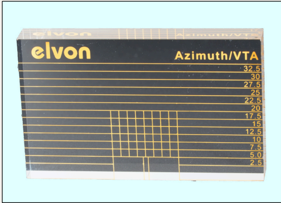
Figure-25: Azimuth and VTA Gauge.
