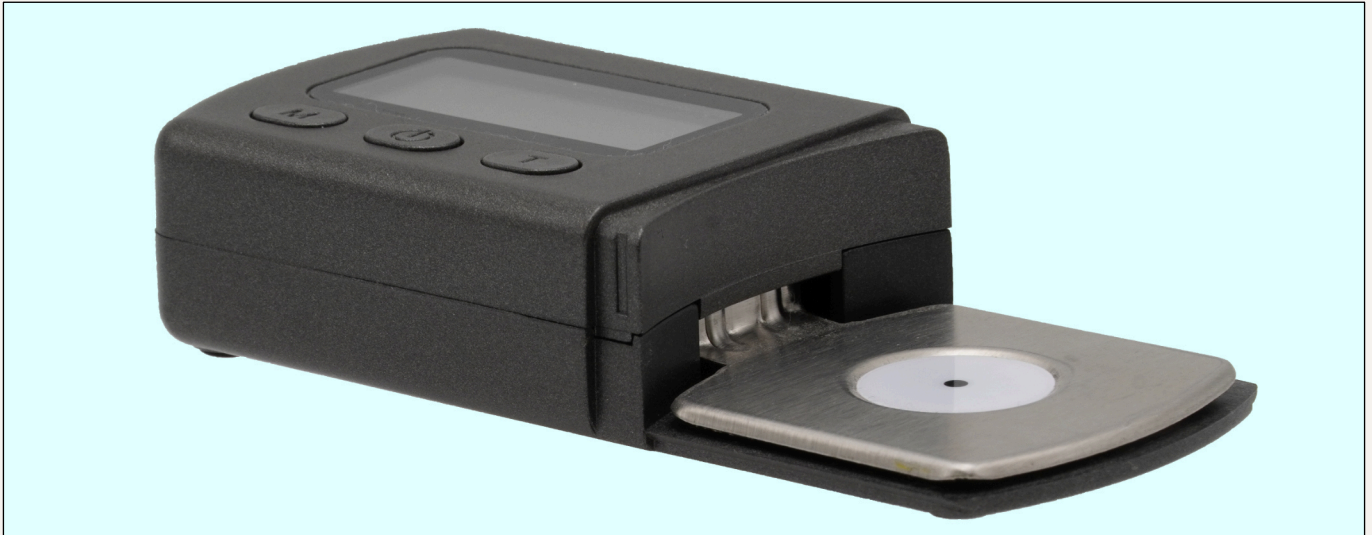
Figure-24: Arm tracking force scales
